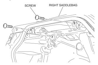
18. Move the right saddlebag catch and remove the plug as shown.
