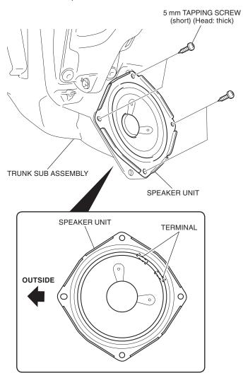
29. Install the left side screw grommet and speaker unit in the same manner as the right side.
