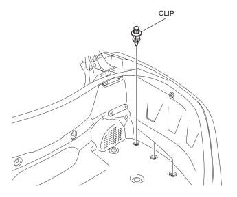
48. Install the trunk front lower panel as shown.
