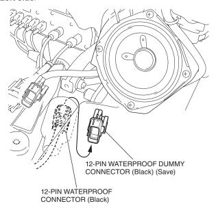
42. Connect the connector as shown.
