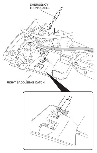
23. Install the radio antenna and right saddlebag catch in the reverse order of removal.
