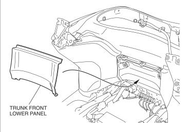
49. Install the 5 mm tapping screws as shown.
