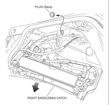
19. Install the emergency trunk cable as shown.
