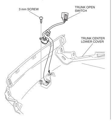
38. Connect the 2-pin black connector and install the trunk center lower cover as shown.
