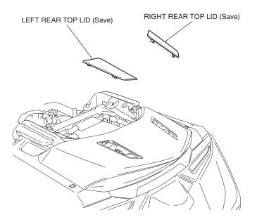
8. Remove the parts as shown.
